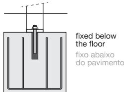
**LF3.1** anchored directly on the concrete foundation
