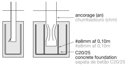
**LF3.5** anchored directly on the concrete foundation
